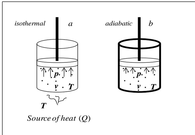
**Fig.2: The gas in the vessels, when expanding, generates mechanical work**
