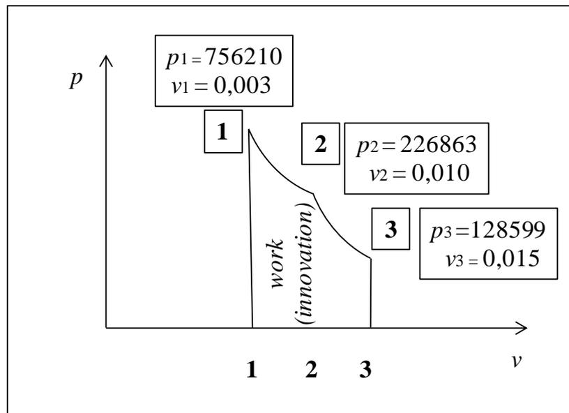
**Fig.3: The area under the curves is the amount of mechanical work from a system operating from 1 to 2 isothermally and from 2 to 3 adiabatically**
