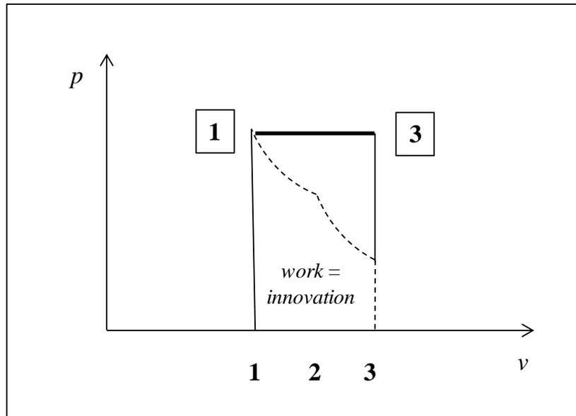
**Fig.5: Transformation at constant pressure. To accomplish the work, more heat than that required by a isothermal is required. In this case, 3970 versus 919 Joule. The internal Energy increases by 1789 joule ( $\Delta U = (Q - W) = 3970 - 2181$ )**
